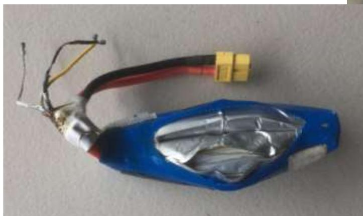
batteries which had then shorted out. The insulation was melted, the battery swelled almost to bursting and a hole melted through the plastic bag. This was potentially a very serious incident as it could have resulted in a car fire, or worse a house fire. Always remember that Lipos store a lot of energy and if damaged can cause a serious napalm like incendiary fire. This was a near miss and whoever was responsible should carefully think about their actions.
