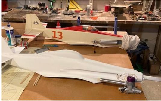
*"The first photo shows my completed little Toni fuse in the background powered by a reasonably tame Irvine 40. The fuselage in front is another little Toni which will house a rather hot OS 46 VX motor capable of close to 30000 rpm. I got a couple of coats of undercoat on before I ran out of paint and no ability to purchase more.*
