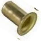
Many people make mistakes when mounting servos that can lead to servo damage, premature servo failure, or other problems. When installing the servos the brass eyelets install from the bottom of the rubber grommet, and then the screw is tightened to where it just touches the top of the rubber grommet. The purpose of the rubber grommet is to isolate the
