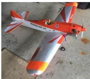
**Rambler 30** – this is from a “the Worlds Models” kit. Span 1450mm<sup>2</sup>. Fitted with OS Max FS46 (ballraced, rear needle valve). Semi-symmetrical airfoil. Servos are a mix of Futaba S3001 and S3003. Needs receiver and battery and a little TLC. The carburettor is damaged – needs new carb or motor.
