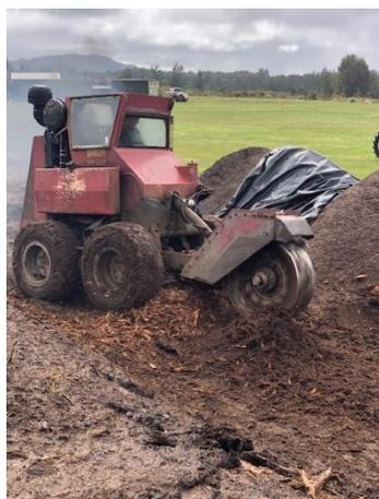
Our carpark earthworks have uncovered a couple of ancient stumps. Rather than incur the cost of digging them out with an excavator, we have engaged a stump grinder to machine them down below ground level. All went well until the machine got stuck and Roger had to use our old tractor to tow him out. Removal of these stumps will enable our contractor to complete the carpark job, hopefully in the next couple of weeks.
