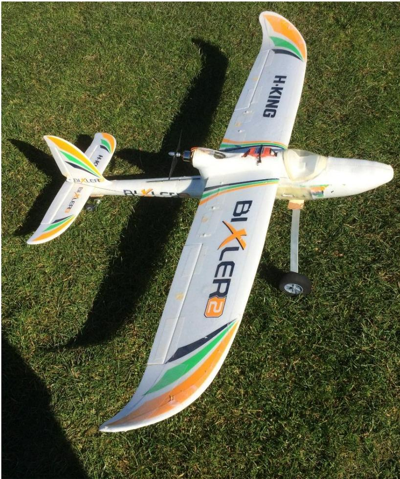
Could this be the ultimate trainer ? This is Daryl King's crash test dummy Bixler. Its had lots of use and shows the scars. Its fitted with uprated motor/ ESC and a taildragger U/C with steerable tailwheel. Its not the prettiest aeroplane, but as a trainer its magic. Almost indestructible, you will never break a propeller, can do endless touch and go landings without stress, and avoids the complications of engine management. Every learner should have one.
